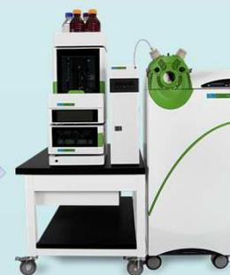
Samples analysis: LC-MS/MS apparatus (Perkin Elmer)
