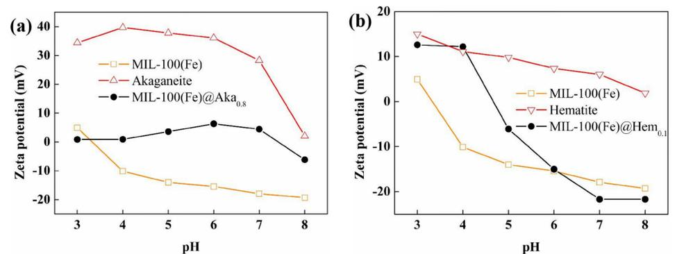
Fig. 2 Zeta potentials against pH for the as-prepared materials
