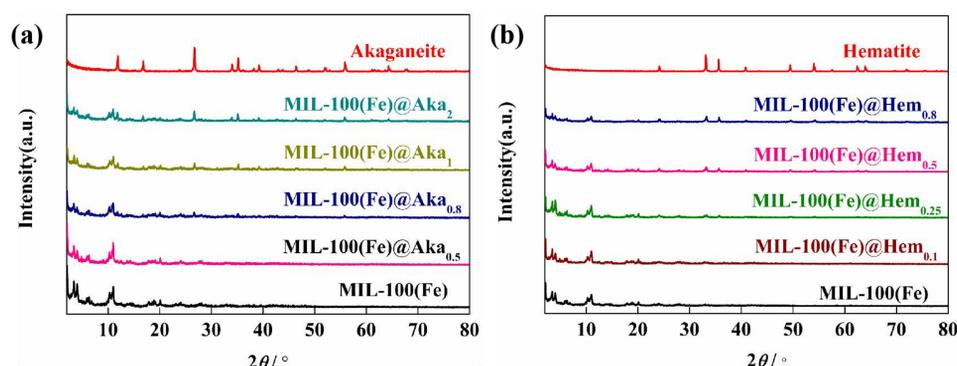
Fig.1 X-ray diffraction patterns of as-prepared materials
