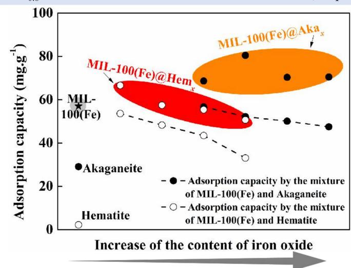
Fig. 3 Adsorption capacities of the as-prepared composites and the mixture of MIL-100(Fe) and akaganeite/hematite at the initial Se(IV) concentration of 200 mg/L
