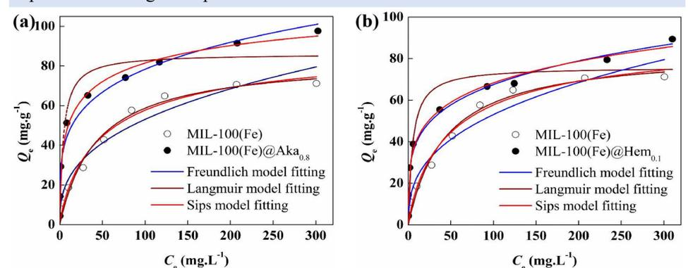
Fig. 4 Isothermal adsorption and fitting curves for Se(IV) by the as-prepared materials
