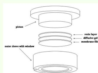
The diffusive gel defines a diffusion domain and the resin gel layer contains a strong binding agent to accumulate the metals. Both gel layers are mounted as discs in a plastic molding and they are covered with a filter, which separates them from the solution.
